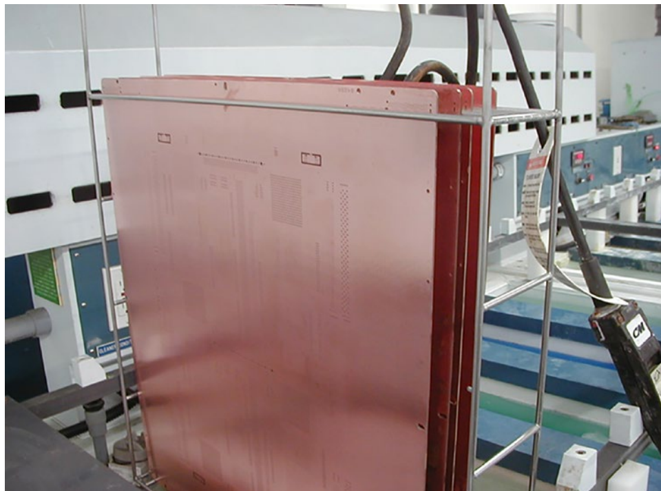
Figure 5: Panels ready for processing. Note the stainless-steel racks are clean and devoid of copper deposits.
