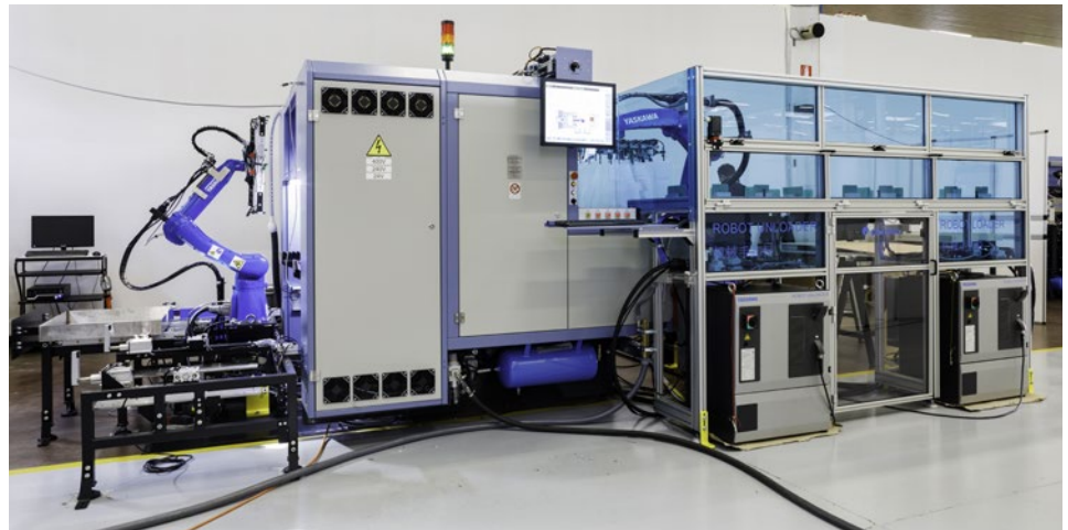
Integrated automation of an X-ray INSPECTA SX using an anthropomorphic robot for front-loading and rear off-loading. Front loader is equipped with buffer stations to handle panel delivery queue while the off-loader takes care of scaling error sorting.
