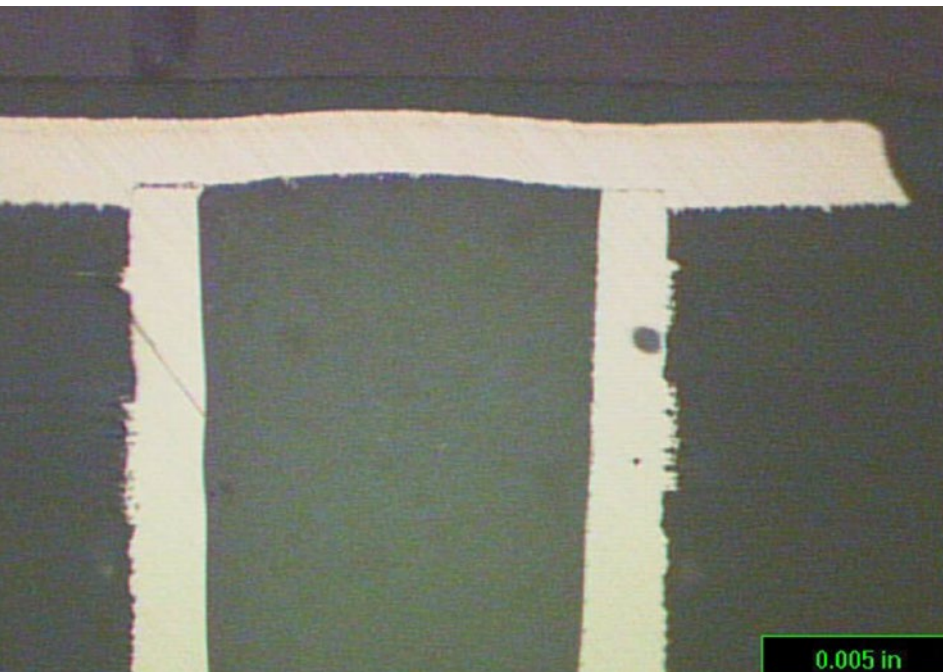
Figure 2: Plated copper separating from filled via due to excessive Z-axis expansion.
