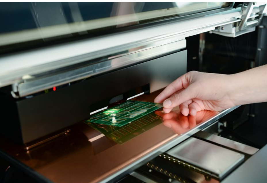
Figure 2: Loading boards into XRF for plating thickness measurement.
